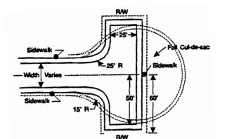
Figure 3: HAMMERHEAD This design is to be used for temporary purposes ONLY. Developers may use this cul-desac design in a phased development where the new street will be expected to continue or connect with other streets in the future.
