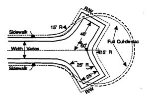
**Figure 4: "Y"** This design is to be used for temporary purposes ONLY. Developers may use this cul-de-sac design in a phased development where the new street will be expected to continue or connect with other streets in the future.
